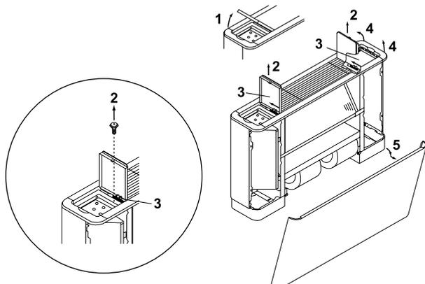
1. Open the lid of control panel (both left and right)
