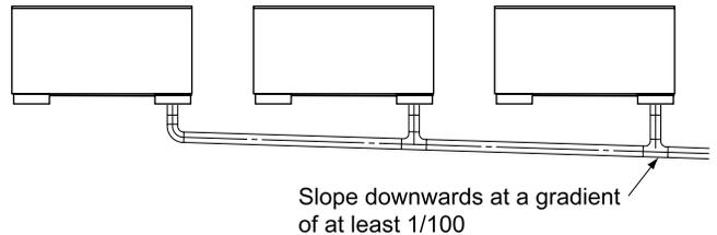
Select converging drain pipes whose gauge is suitable for the operating capacity of the unit.
