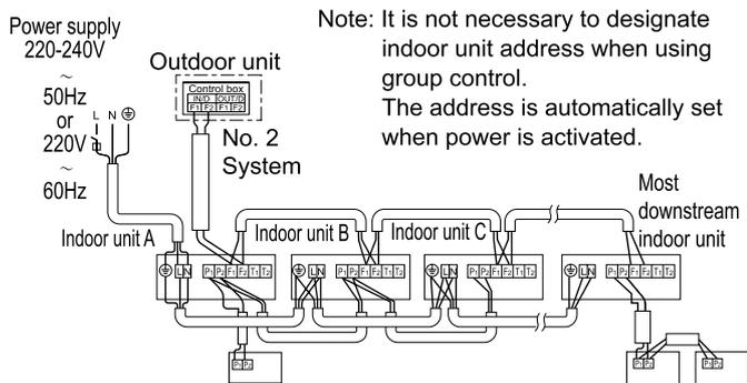
Note: It is not necessary to designate indoor unit address when using group control. The address is automatically set when power is activated.
