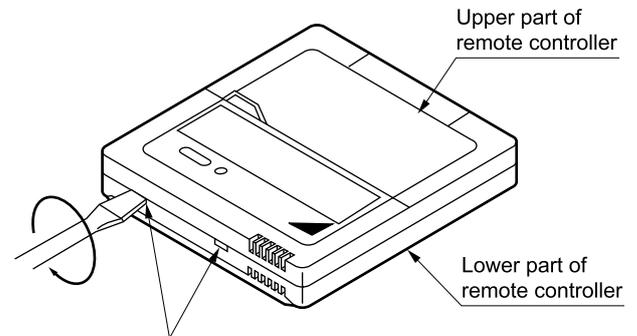
Insert the screwdriver here and gently work off the upper part of remote controller.
