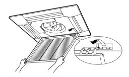
**3. Detach the air filter.** Refer to "HOW TO CLEAN THE AIR FILTER".
