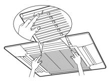
2. Detach the suction grille. Open the suction grille 45 degrees and lift it upward.
