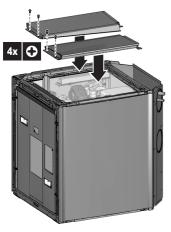
3 Stick the top plate insulation (accessory) at the inside of the top decoration panel according to the figure below.
