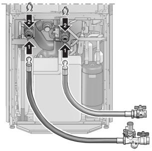
Installation of accessory pipes for refrigerant piping. Depending on left or right connection, different accessory pipes are delivered with the unit (refer to "4. Accessories" on page 4). The refrigerant piping needs to be brazed.
