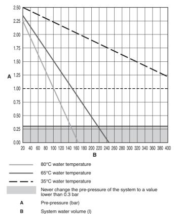
How to check if the pre-pressure of the system needs to be changed:
