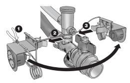
Mounting of the manometer against a wall (the 2 screws are field supply).
