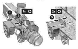
Fix the indoor unit refrigerant connections
