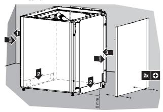
Close the sound panel(s) and decoration panel(s) which will be on the wall side and for which fixation is not possible anymore after the unit is put on its final location.
