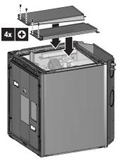
Stick the top plate insulation (accessory) at the inside of the top decoration panel according to the figure below.
