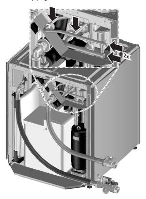
Fixation of piping in case of right connection
