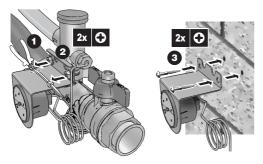
Fix the indoor unit refrigerant connections
