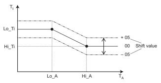
$egin{array}{ll} T_t & \mbox{Target water temperature} \\ T_A & \mbox{Ambient (outdoor) temperature} \\ \mbox{Shift value} & = \mbox{Shift value} \\ \end{array}$
