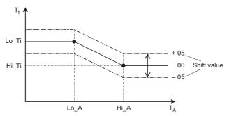
T<sub>t</sub> Target water temperature
