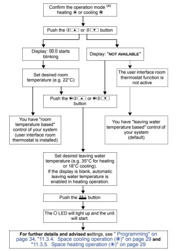
(a) The operation mode can not be selected on the hydrobox. The hydrobox follows the operation mode of the master VRV DX Indoor Unit. Refer to outdoor unit manual for further information
