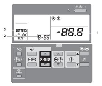
1 Press the substrained button for a minimum of 5 seconds to enter FIELD SET MODE.
