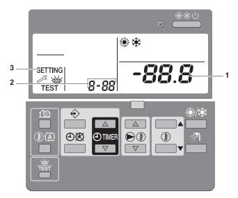
1 Press the button for a minimum of 5 seconds to enter FIELD SET MODE.
