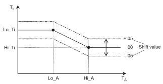
T<sub>t</sub> Target water temperature
