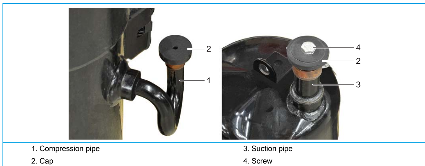
Figure 73 - Installing a new compressor - 1
