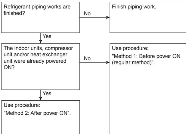
It is very important that all refrigerant piping work is done before the units (compressor unit, heat exchanger unit or indoor units) are powered on.
