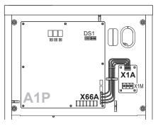
5 Connect the cool/heat selector switch. Tightening torque X1M (A/B/C): 0.53~0.63 N•m
