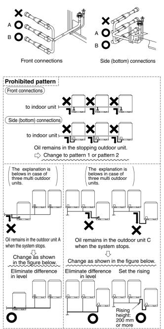
(3) If the piping length between the outdoor units exceeds 2 m, create a rise of 200 mm or more in the gas line under a length of 2 m from the outdoor unit multi connection piping kit.
