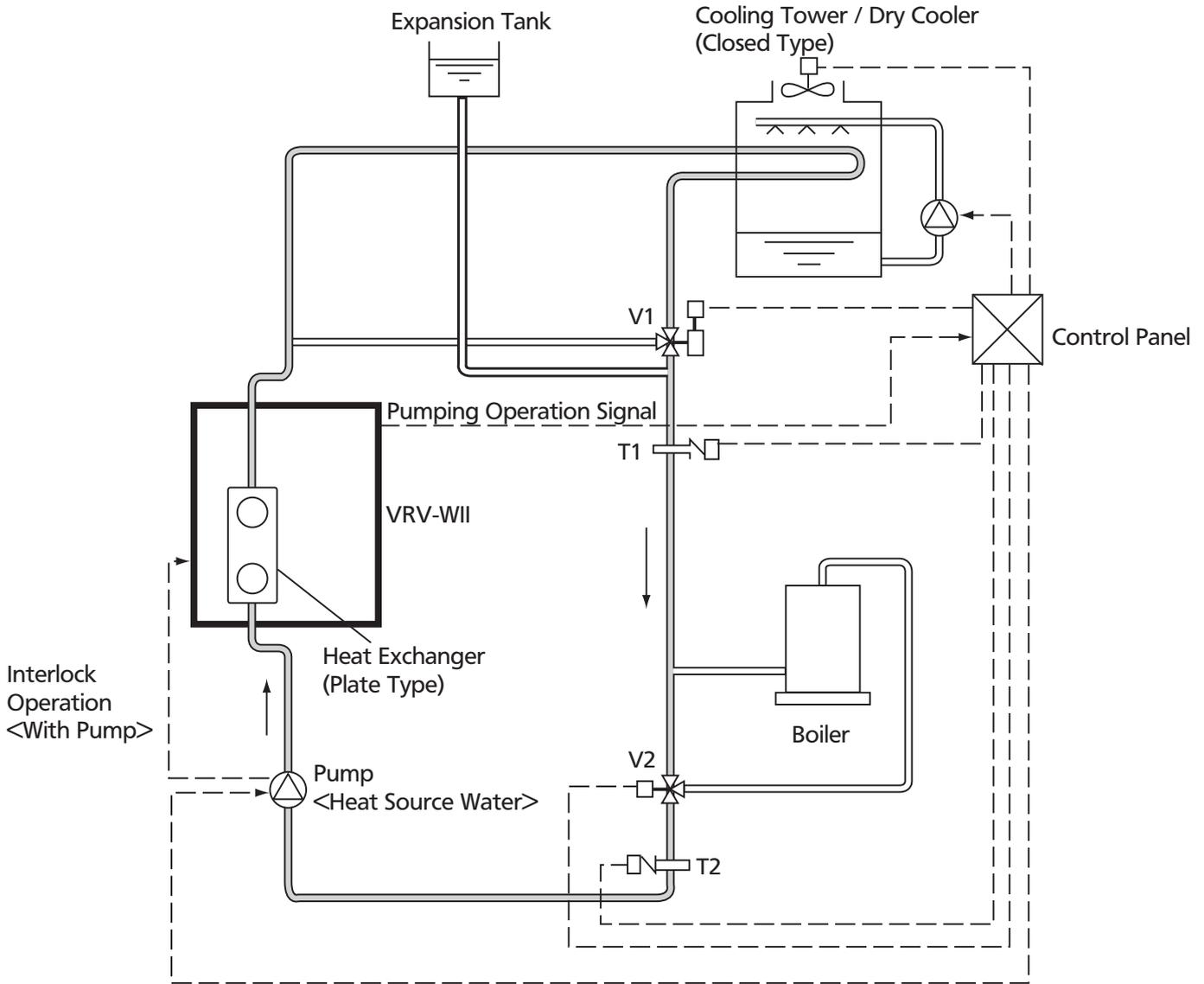
The diagram shows that during summer operating cycles, a drop in cooling water temperature below pre set temperature level T1 causes 3-way valve bypass V1 to open. This bypass closes once more when T1 is exceeded, reducing the temperature by allowing an increased flow of water to the cooling tower. On/off control of pump and fan in closed cooling tower circuits is also provided by 3-way valve, V1.
