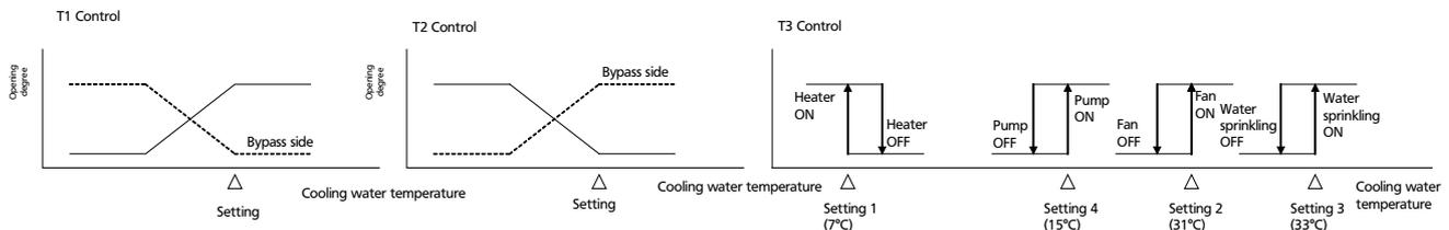
\*If freezing is expected to occur, install the freezing protection heater or drain water from the water sprinkling side. (If water is drained from the water sprinkling side, pay attention so that loads will never be applied to cooling mainly.)
