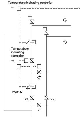
Typical modification to Part B (Three-way valve → Two-way valve)
