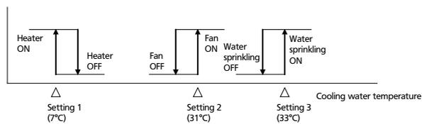
\*If freezing is expected to occur, install the freezing protection heater or drain water from the water sprinkling side.
