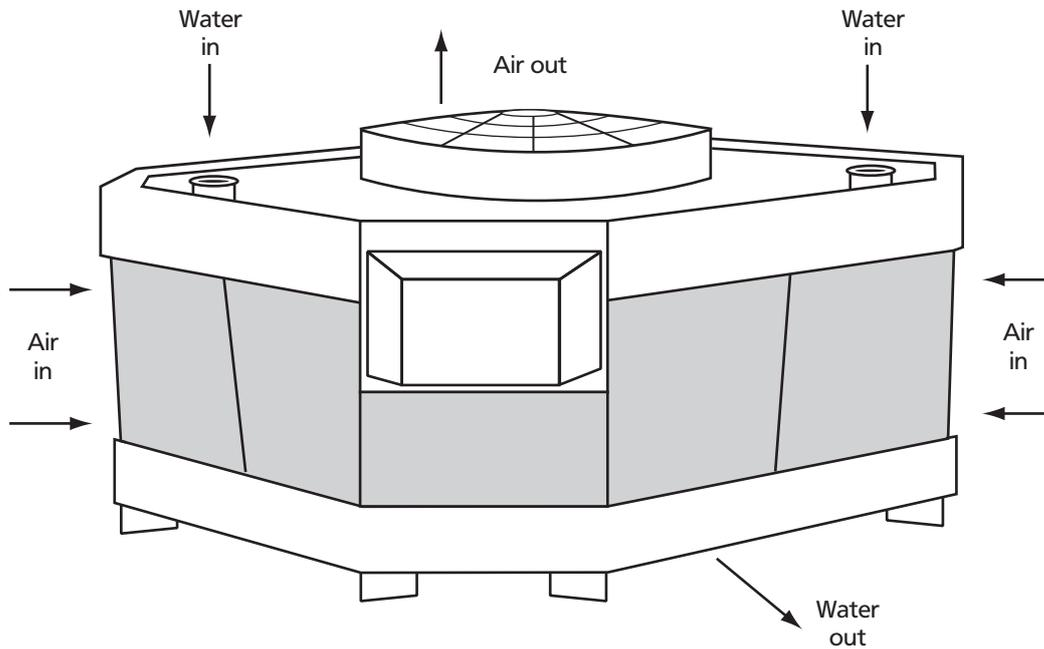
Large propeller fans on the air discharge or the top of the tower **draw air counter flow or cross flow** to the condenser water. Due to the higher discharge velocities they are less susceptible to short air circuits or recirculation. Noise levels are higher due to the low frequency noise associated with propeller and axial fans.
