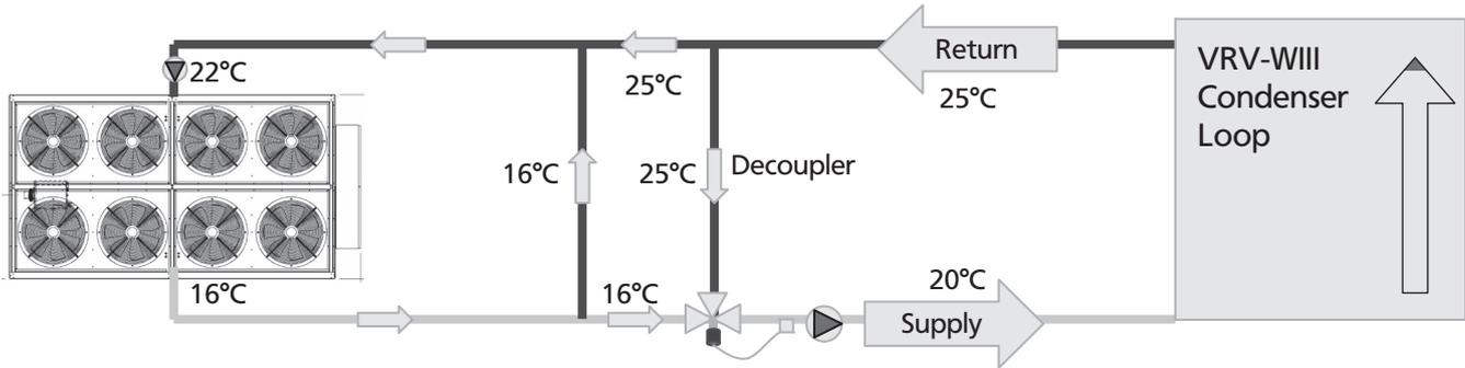
To ensure maximum operating efficiency of the heat pump chiller, the following data represents the optimum selection point when using the above configuration: -
