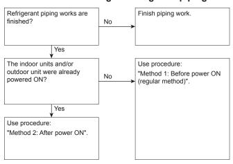
It is very important that all refrigerant piping work is done before the units (outdoor or indoor) are powered on.
