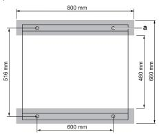
Fasten the unit in place using four foundation bolts M12. It is best to screw in the foundation bolts until their length remains 20 mm above the foundation surface.
