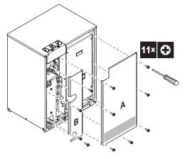
Once the front plate A is open, the electrical component box can be accessed. See "6.2.2 To open the electrical component box of the outdoor unit" on page 23.
