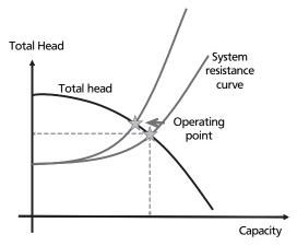
The pump selection can be carried out through calculation or by use of the pump selection chart:
