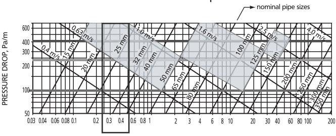
Fig. 1 VOLUMETRIC FLOW RATE, L/s
