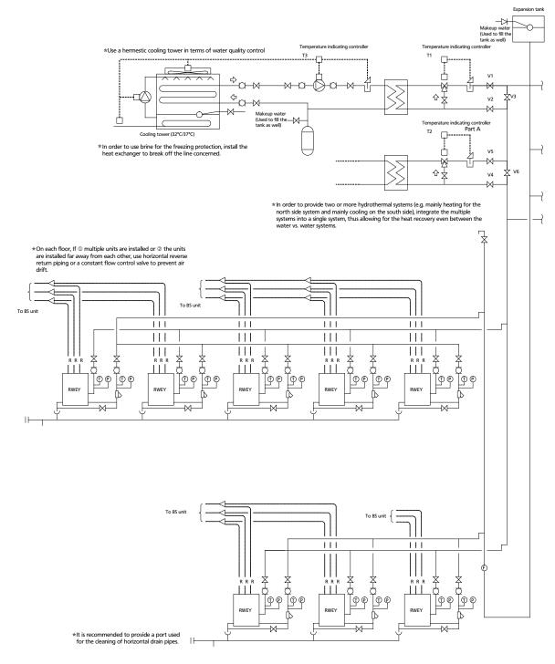
\*For RWEY models, provide interlock with the flow switch. (Through the pump operation signal, an operative flow switch is recommended.)
