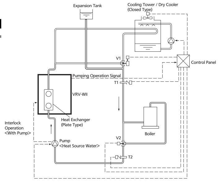
During winter operation, water circuit temperature T2 is maintained by circulating water through the boiler (or similar) via valve V2, which shuts off immediately the pre set temperature is achieved.
