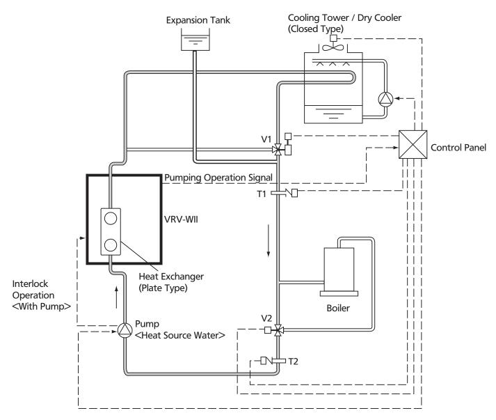
The diagram shows that during summer operating cycles, a drop in cooling water temperature below pre set temperature level T1 causes 3-way valve bypass V1 to open. This bypass closes once more when T1 is exceeded, reducing the temperature by allowing an increased flow of water to the cooling tower. On/off control of pump and fan in closed cooling tower circuits is also provided by 3-way valve, V1.
