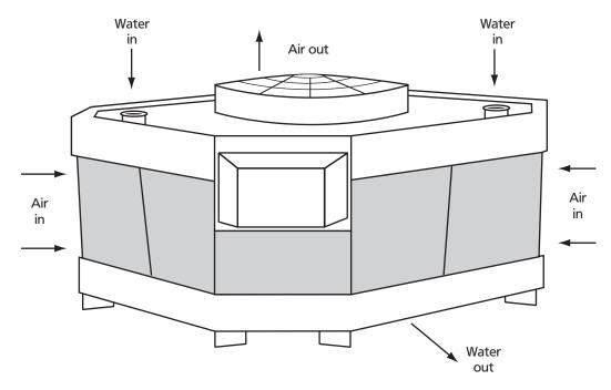
Large propeller fans on the air discharge or the top of the tower **draw air counter flow or cross flow** to the condenser water. Due to the higher discharge velocities they are less susceptible to short air circuits or recirculation. Noise levels are higher due to the low frequency noise associated with propeller and axial fans.
