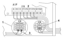
1 Pump operation output terminal (X2M) For linking water pump operation to system operation, the water pump operation circuit wiring is to be connected to terminals 1 and 2 (X2M). Contact specifications: 220 VAC, 3 mA-0.5 A
