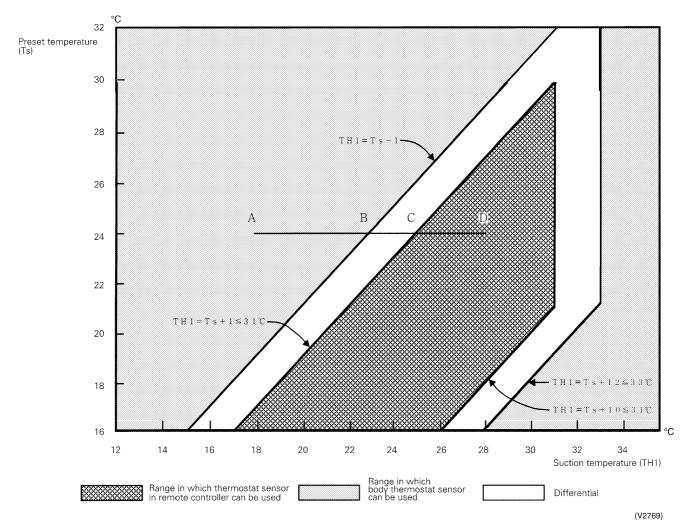
**Ex:** When heating Assuming the preset temperature in the figure above is 24°C, and the suction temperature has changed from 18°C to 28°C (A  $\rightarrow$  D):
