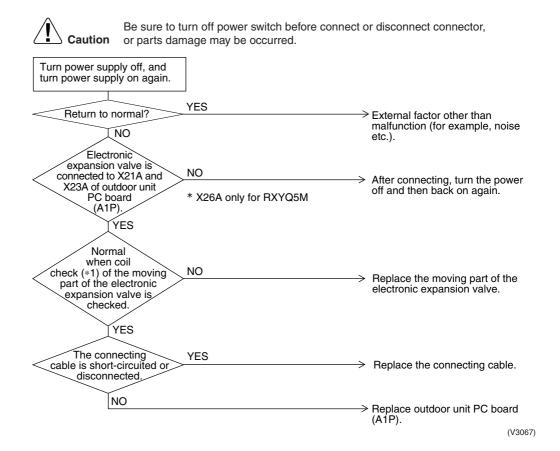
\*Make measurement of resistance between the connector pins, and then make sure the resistance falls in the range of 40 to  $50\Omega$ .
