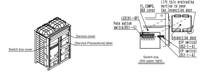
Caution When the 400 volt power supply is applyed to "N" phase by mistake, replace Inverter P.C.B (A2P) and control transformer (T1R, T2R) in switch box together.
