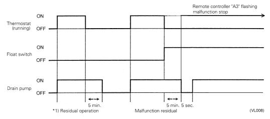
\* 1. The objective of residual operation is to completely drain any moisture adhering to the fin of the indoor unit heat exchanger when the thermostat goes off during cooling operation.
