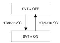
HTdi: Correction value of the discharge pipe temperature on the INV compressor.
