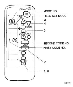
1. When in the normal mode, push the " button for 4 seconds or more, and operation then enters the "field set mode."
