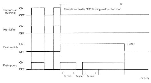
During heating operation, if the float switch is not reset even after the 5 minutes operation, 5 seconds stop, 5 minutes operation cycle ends, operation continues until the switch is reset.
