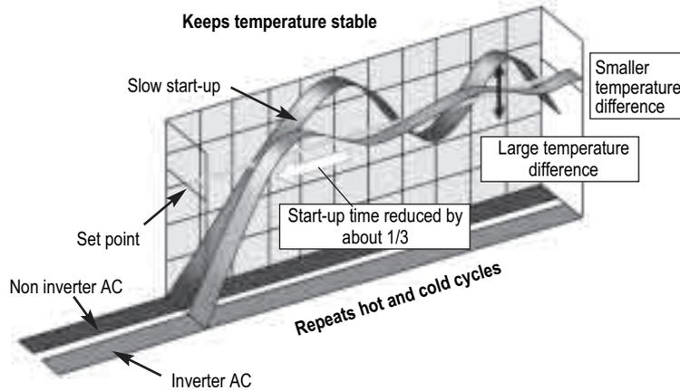
The thermostat can control stable room temperature at  $\pm 0.5^{\circ}\text{C}$  from set point.
