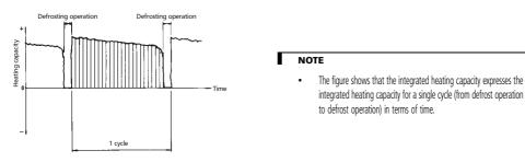
3 Please note that when there is an accumulation of snow against the outside surface of the outdoor unit heat exchanger, there will always be a temporary reduction in capacity although this will, of course, vary in degree in accordance with a number of other factors such as the outdoor temperature ( CDB), relative humidity (RH) and the amount of frosting which occurs.
