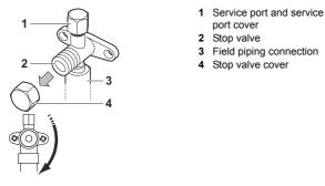
2 Connect the vacuuming/recovery unit to service ports of all stop valves.
