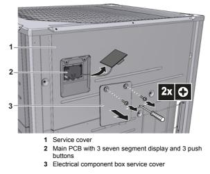
Operate the switches and push buttons with an insulated stick (such as a closed ball-point pen) to avoid touching of live parts.
