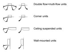
For the following conditions, a micro computer controls the air flow direction which may be different from the display.
