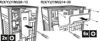
For service purposes, the push buttons on the main PCB need to be accessed. To access these push buttons, the electrical component box cover does not need to be opened. See "13. Making field settings" on page 29.
