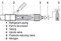
Do not use anti-oxidants when brazing the pipe joints. Residue can clog pipes and break equipment:
