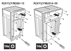
Once the front plates open, the electrical component box can be accessed by removing the electrical component box cover as follows.
