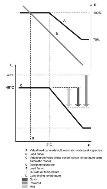
Example: Automatic mode during heating
