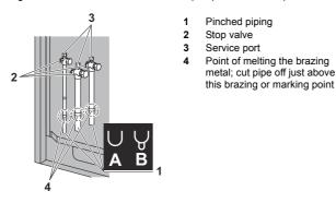
**6** For equalizing gas and gas stop valves, cut off the lower part of the smaller pinched piping with an appropriate tool (e.g., pipe cutter, a pair of nippers, ...). Let the remaining oil drip out in case the recovery was not complete.
