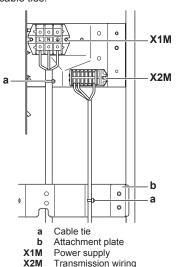
6 Route the wiring through the frame and connect it to it.
