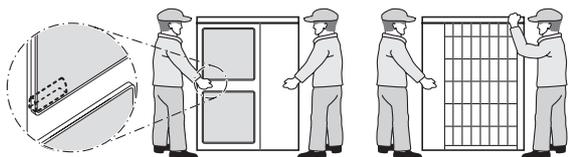
Place your hands on the corner instead of holding the suction inlet in the side of the casing, otherwise the casing could be deformed.
